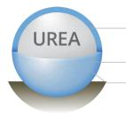
**Thickness of coating** determines longevity from 60 to 180 days per application
